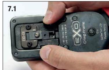
8) Replacing EXO Die™ Same as removing the die set BUT in reverse.
